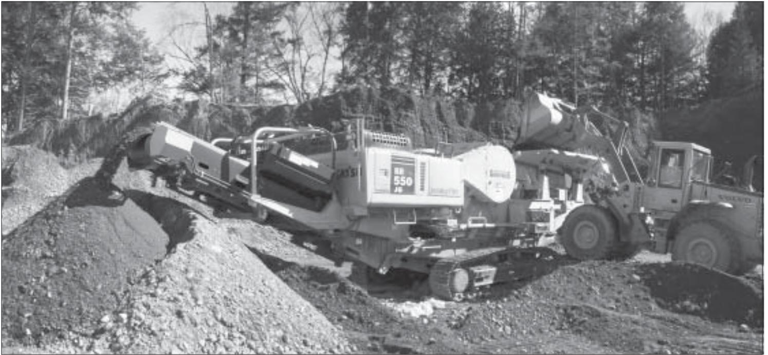
*Portable crusher manufactures aggregates for LP expansion project.*
