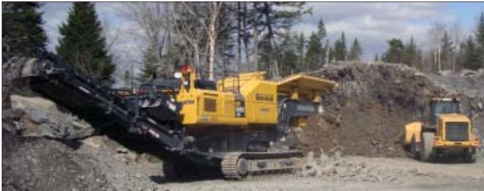
*Komatsu BR580 jaw crusher makes type D gravel.*
