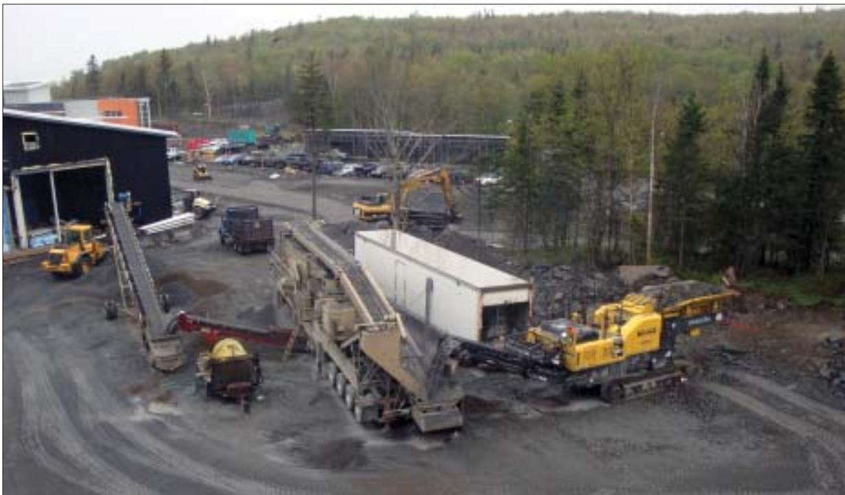
*Komatsu BR580 jaw crusher and JCI cone crusher make type A gravel.*
